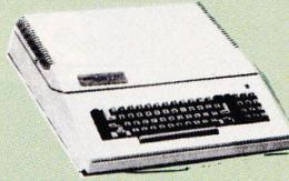
The Franklin ACE 1000 includes 64K RAM, upper/lower case character set (40 columns), hi-res graphics, numeric keypad, 8 peripheral slots, joystick/paddle connectors, and a built-in cooling fan. The Franklin ACE 1000 has full hardware/software compatibility with all existing Apple II® products.
